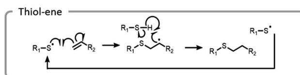
Fig. 12 Mechanism of thiol-ene catalytic reaction.
