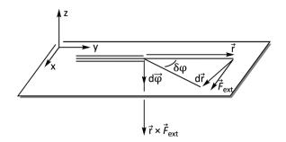
Fig. 2 Vector model of alkyne bending used for the extension of the COGEF approach towards bending forces.
