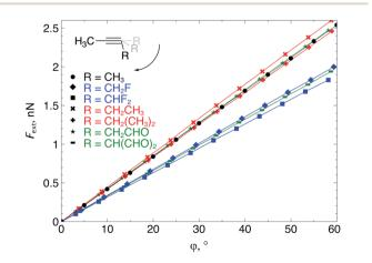
Fig. 4 The required bending force in acetylenes increases linearly with the bending angle  $\varphi$ , according to eqn (5) but clearly varies upon substitution.
