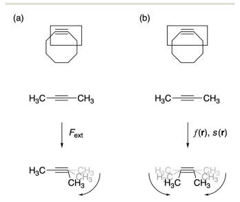
Fig. 3 (a) The bending force was calculated by constraining one bond angle; (b) the reactivity of the triple bond in cyclic alkynes was modeled by constraining both angles around the triple bond.
