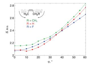
Fig. 8 The global softness of a 2-butyne fragment starts to increase when the triple bond is bent to an angle of  $15^\circ$  due to an increase of the in-plane  $\pi\text{-HOMO}$  energy and a decrease of the in-plane  $\pi\text{-LUMO}$  energy.
