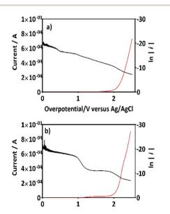
Fig. 11 The variation of current as a function of the overpotential ( $\eta$ ) for BDD in (a) 0.5 M Na<sub>2</sub>SO<sub>4</sub> solution and (b) 0.5 M Na<sub>2</sub>SO<sub>4</sub> + 100 ppm 2,4-DNa (pH 3) solution at 10 mV s<sup>-1</sup> and 298 K. Tafel curves are included for each one of the cases plotting ln(i) against  $\eta$  (black curves).
