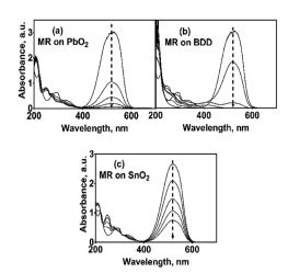
Fig. 5 UV-vis spectra for 20 mg  $\rm L^{-1}$  MR solutions in 0.5 M  $\rm H_2SO_4$  electrolyzed at 30 mA cm<sup>-2</sup> and 298 K, as a function of the electrolysis time and the material of anode: (a) Pb/PbO<sub>2</sub>, (b) Si/BDD and (c) Ti/Sb-doped SnO<sub>2</sub>.
