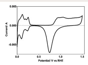
Fig. 1 Voltammogram of the Pt electrode used as cathode, recorded in 0.5 M  $H_2SO_4$  as supporting electrolyte at v=50 mV s<sup>-1</sup> and at 298 K.
