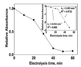
Fig. 9 Plot of the relative absorbance at 285 nm of 2,4-DNa as a function of the electrolysis time for the electrolysis of a solution containing 100 mg  $\rm L^{-1}$  2,4-DNa in 0.5 M Na<sub>2</sub>SO<sub>4</sub> at 30 mA cm<sup>-2</sup> and 298 K on Si/BDD anode. Inset shows the corresponding pseudo-first order graphic.
