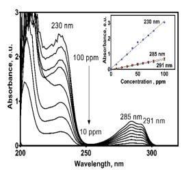
Fig. 3 UV absorption spectra of 2,4-DNa in 0.5 M Na<sub>2</sub>SO<sub>4</sub> (pH 3) solution as a function of 2,4-DNa concentration in the range of 10–100 mg  $\rm L^{-1}$ . Inset: Beer law applied to each one of absorption bands considered.
