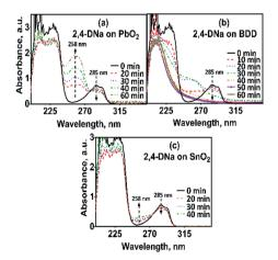
Fig. 8 UV spectra for 100 mg  $\rm L^{-1}$  2,4-DNa solutions in 0.5 M Na<sub>2</sub>SO<sub>4</sub> electrolyzed at 30 mA cm<sup>-2</sup> and 298 K, as a function of the electrolysis time and the material of anode: (a) Pb/PbO<sub>2</sub>, (b) Si/BDD and (c) Ti/Sb-doped SnO<sub>2</sub>.
