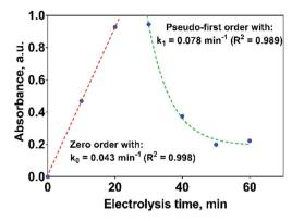
Fig. 10 Kinetic parameters for the formation and consumption of 2,4-DP as first reaction intermediate on the Si/BDD anode in  $0.5 \text{ M Na}_2\text{SO}_4$  + 100 ppm 2,4-DNa solution at 30 mA cm<sup>-2</sup> and 298 K.
