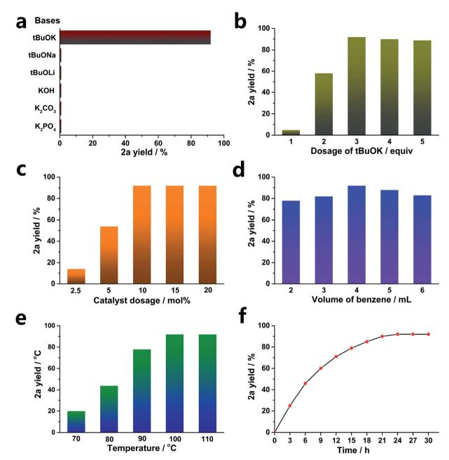
Fig. 1 SOM-catalyzed C-H arylation of benzene with iodobenzene. (a) Effects of bases. (b) Dosage of <sup>t</sup>BuOK, (c) catalyst dosage, (d) volume of benzene, (e) effects of temperature, (f) dynamic tests. Standard reaction conditions: PhI 0.4 mmol, benzene 4 mL, <sup>t</sup>BuOK 1.2 mmol, SOM 10 mol%, 100 °C, 24 h, unless otherwise stated; yields were determined by GC using dodecane as an internal standard.
