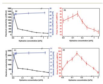
Fig. 3 TE properties of PEDOT:PSS films as a function of the hydrazine concentration. (a and b) Formic acid  $\times$  1 time and hydrazine  $\times$  1 time; (c and d) formic acid  $\times$  3 times and hydrazine  $\times$  1 time.
