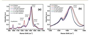
Fig. 7 (a) Raman spectra of the PEDOT:PSS films before and after treatment with formic acid and formic acid—hydrazine. (b) The zoomin spectra for the wavenumbers ranging from 1300 to 1500 cm<sup>-1</sup>.
