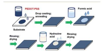
Fig. 1 Schematic of preparation and sequential post-treatment of PEDOT: PSS films with formic acid and hydrazine.
