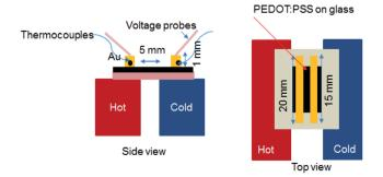
Fig. 2 Schematic illustrations of the setup of S measurement and the electrode geometry. Side view (left) and top view (right).
