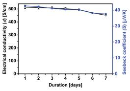
Fig. 10 The effect of stability of  $\sigma$  and S at the optimum doping level with formic acid-0.15 wt% hydrazine treatment of PEDOT:PSS film as a function of exposure time (humidity: 75%; temperature: 70 °C).
