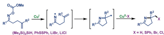
Scheme 4 Narasaka's copper-catalyzed imino-functionalization of \gamma,\delta -unsaturated oxime esters.
