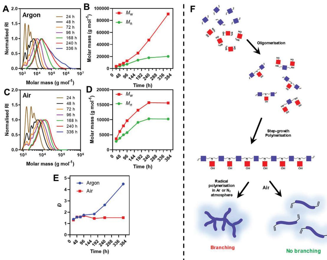
**Fig. 2** (A and C) DMF-SEC chromatograms and (B and D) molecular weight evolution of pABOL at  $[M] = 0.60$  M,  $T = 45$   $^{\circ}\text{C}$  polymerisation in an argon or air atmosphere. (E) Evolution of dispersity over time for pABOL. (F) Schematic representation of step-growth polymerisation and subsequent radical polymerisation leading to branching under inert conditions and inhibition of radical polymerisation under air.
