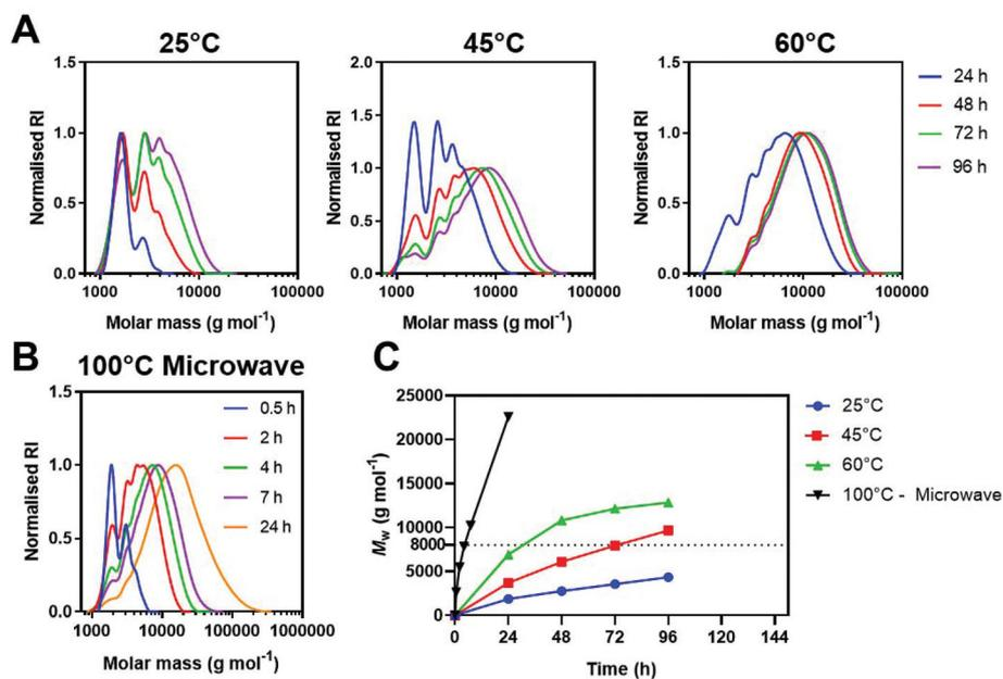
Fig. 3 (A and B) DMF-SEC chromatograms and (C) molecular weight evolution of pABOL at  $[M] = 0.60 \text{ M}$  and air atmosphere at 25 °C, 45 °C and 60 °C under conventional heating at 100 °C under using microwave assisted heating.
