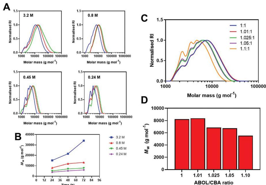
Fig. 4 (A) DMF-SEC chromatograms and (B) molecular weight evolution of ABOL + CBA polymerisations at 60 °C and an air atmosphere at  $[M] = 3.2, 0.8, 0.45$  and  $0.24$  M. (C) DMF-SEC chromatograms and (D)  $M_{w,SEC}$  of final polymers after 48 h reaction between CBA and ABOL at different ABOL/CBA ratios. Reactions were performed at 60 °C and an air atmosphere at  $[M] = 0.60$  M.
