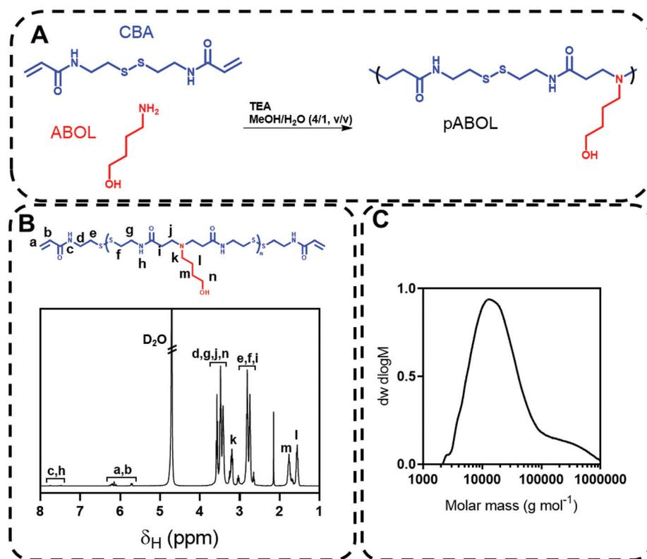
**Fig. 1** (A) Synthetic scheme for step-growth Michael-addition polymerisation of *N,N'*-cystaminebisacrylamide and 4-amino-1-butanol to produce pABOL; (B) <sup>1</sup>H NMR spectrum of pABOL; (C) size exclusion chromatogram of product obtained via 'conventional' synthesis.
