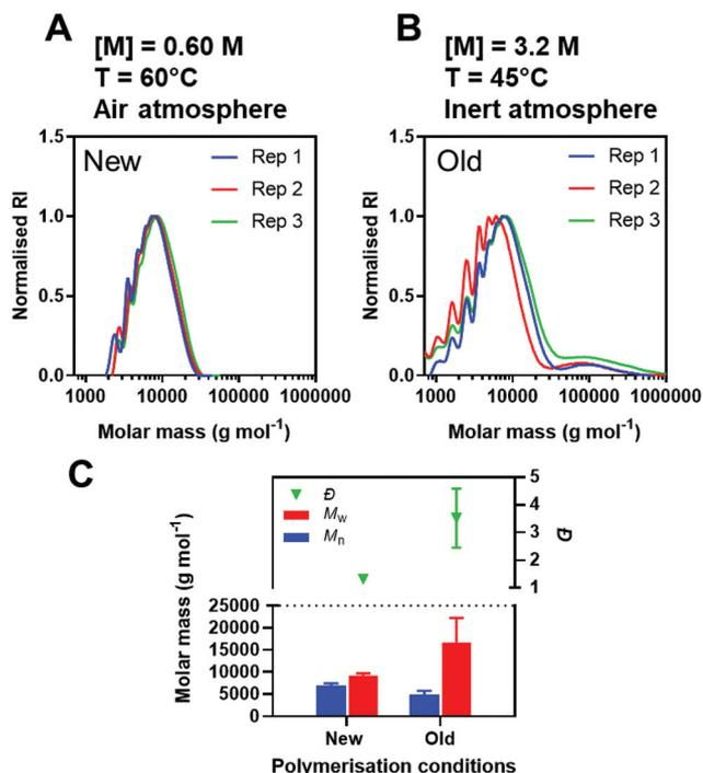
Fig. 5 (A and B) DMF-SEC chromatograms and (C)  $M_w$  of final polymers after 48 h reaction between CBA and ABOL performed in triplicate. Reactions were performed at 60 °C, [M] = 0.60 M and an air atmosphere compared to 45 °C, [M] = 3.2 M and an argon atmosphere.
