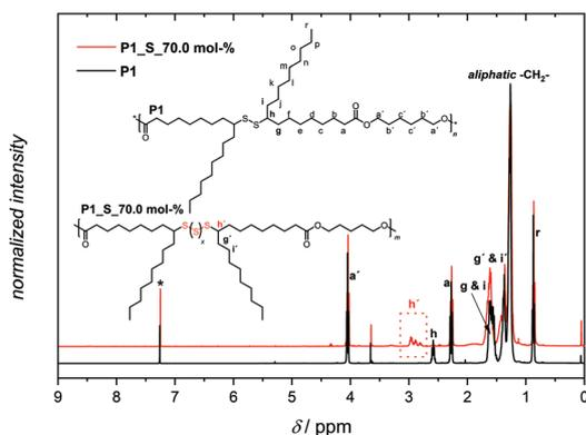
Fig. 3 Analysis of **P1** and **P1\_S\_70.0 mol%** by  $^1\text{H}$  NMR spectroscopy, indicating the success of each transformation, the synthesis of the parent polymer **P1** and the subsequent organocatalytic sulfur exchange reaction with 70.0 mol% elemental sulfur added incrementally.
