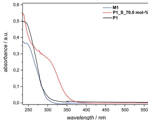
Fig. 5 UV-Vis spectra of **M1**, **P1** and **P1\_S\_70.0 mol%**. Sample concentrations were  $1.23 \times 10^{-5}$  mmol mL $^{-1}$  (for **M1**) and  $6.25 \times 10^{-2}$  mg mL $^{-1}$  (for **P1** and **P1\_S\_70.0 mol%**.) in THF. Solvent cut-off wavelengths  $\lambda_0$ : 215 ( $\lambda_{\text{max}}$ : 220 nm in THF). For details, refer to the main text and the ESI.†
