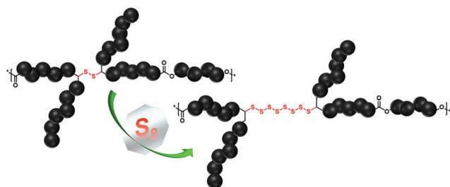
**Fig. 1** Organocatalytically triggered reaction of S<sub>8</sub> with secondary disulfide bonds, which are placed in each repeating unit of the sustainable polyester derivative, to deliver high sulfur content linear polyester derivatives with tailored properties.
