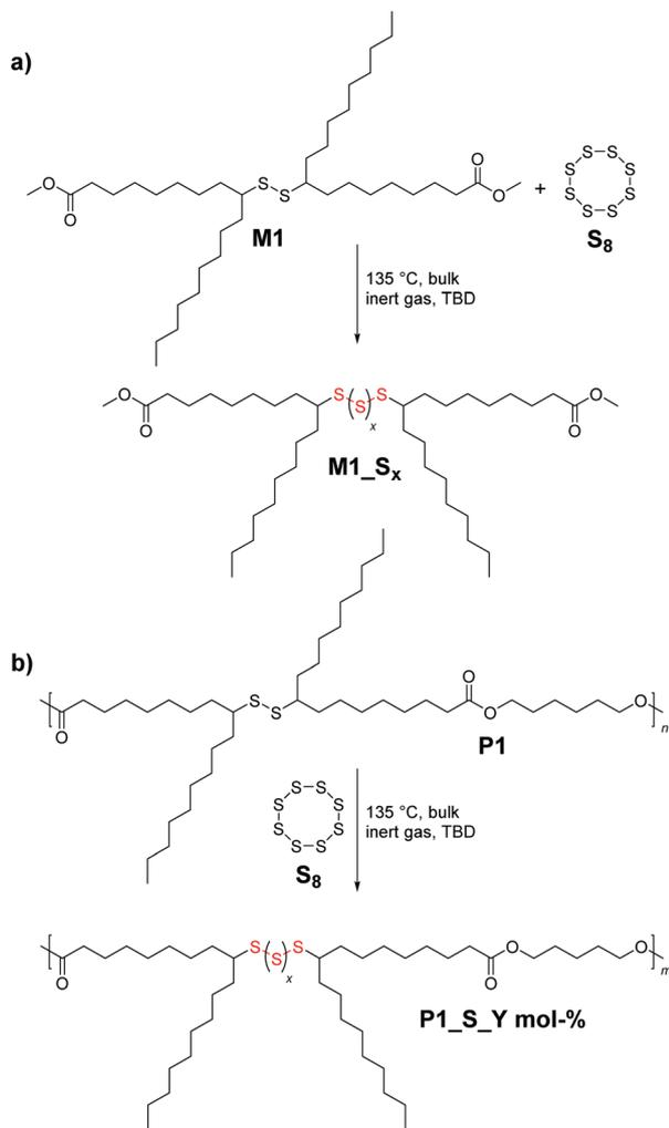
**Scheme 3** The organocatalytically (*i.e.* TBD) triggered sulfur exchange reaction between  $S_8$  and the secondary disulfide bonds of: (a) monomer **M1** to synthesize a proof-of-concept molecule **M1<sub>S<sub>x</sub></sub>** and (b) polymer **P1** to deliver **P1<sub>S<sub>Y</sub> mol-%</sub>**, respectively. "x" indicates the number of sulfur atoms introduced after the sulfur exchange reaction and "Y" stands for the loading of  $S_8$  (in mol%) during the reaction.
