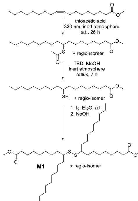
**Scheme 1** Synthetic route for the preparation of renewable monomer **M1** (dimethyl 9(10),9'(10')-dithiodistearate) bearing secondary disulfide groups, suitable to undergo the organocatalytic sulfur exchange reaction.
