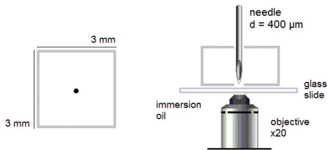
**Fig. 1** Schematic depiction of the experimental setup for analysis with CLSM showing the needle-punctured rectangular hydrogel sample and wet mounting onto glass slide for imaging with an inverted microscope.
