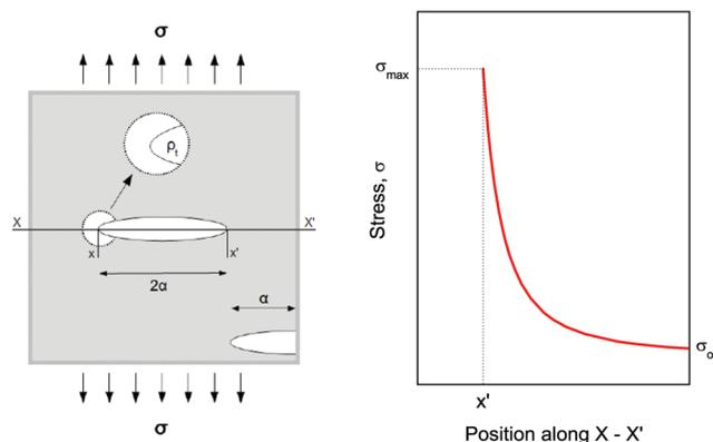
**Fig. 2** Surface and internal flaws in a plate and stress profile with distance along the axis. Since all materials tend to contain flaws, any externally applied force would not be uniformly distributed throughout their structure. Internal cracks and voids, thus, have the role of stress concentrators.
