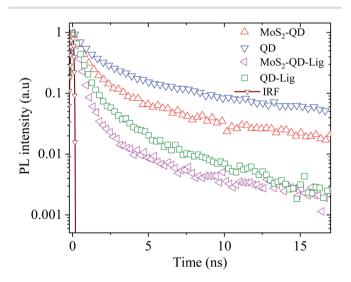
Fig. 4 TRPL data of the QD-MoS<sub>2</sub> monolayer hetero-structure along with the instrument response function (IRF). All data were fitted with bi-exponential functions as discussed in the ESI.†
