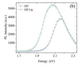
Fig. 3 PL data of (a) the QD $-MoS_2$  monolayer hetero-structure before and after ligand exchange while (b) shows the same on  $SiO_2$  before and after ligand exchange.
