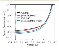
Fig. 4 J-V characteristics of the fabricated OSCs under illumination with an intensity of 75 mW cm $^{-2}$ . The OSCs were illuminated at the normal incidence angle.
