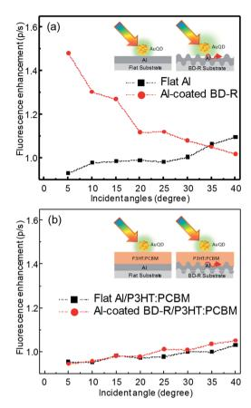
Fig. 7 (a) Fluorescence enhancement (p/s) spectra of G-AuQDs deposited on a flat Al film and an Al-coated BD-R. (b) Fluorescence enhancement (p/s) spectra of G-AuQDs deposited on a flat Al/ P3HT:PCBM film and an Al-coated BD-R/P3HT:PCBM film. The fluorescence of G-AuQDs at 530 nm was recorded under illumination with a wavelength of 350-500 nm.
