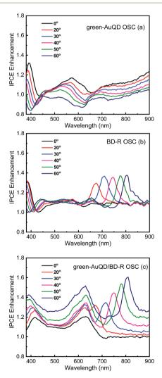
Fig. 5 IPCE enhancement spectra of green-AuQD/BD-R OSCs under the irradiation of non-polarized light at various angles of incidence. (a) Green-AuQDs OSC, (b) BD-R OSC and (c) green-AuQD/BD-R OSC.
