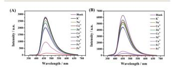
Fig. 9 Fluorescence spectra of (A) CDs-2 and (B) CDs-3 with different metal salts including  $\rm K^+, Na^+, Zn^{2+}, Ca^{2+}, Co^{2+}, Ni^{2+}, Cu^{2+}, Fe^{2+},$  and  $\rm Fe^{3+}.$
