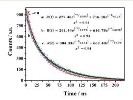
Fig. 6 Fluorescence lifetime decay profiles of CDs-1 (a), CDs-2 (b), and CDs-3 (c).
