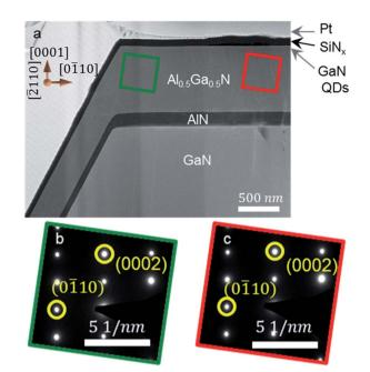
Fig. 4 (a) Cross-sectional view HAADF STEM image taken near the boundary region of the truncated pyramid structure. (b and c) SAD pattern images of the  $Al_xGa_{1-x}N$  layers below B- and P-QDs, respectively. Note that the  $SiN_x$  and Pt layers are deposited to protect the GaN QDs layers when preparing a STEM specimen.
