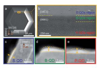
Fig. 2 (a) Top-view SEM image of a single truncated pyramid. (b) Highresolution SEM image of the boundary between (0001) polar and {1011} semipolar facets. (c-e) HAADF STEM images of S-, B-, and P-QDs on the surface of the truncated pyramid, respectively.
