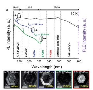
Fig. 3 (a) PL and PLE spectra at 10 K. The black line shows the broadband UV emission spectrum. Blue and green lines indicate the PLE intensity of S- and B-QDs, respectively. DAP stands for donor-toacceptor pair. (b-f) Low-temperature (10 K) monochromatic CL images of a single truncated pyramid measured at 280 nm, 293 nm, 313 nm, 330 nm, and 340 nm, respectively (scale bars: 10 μm).
