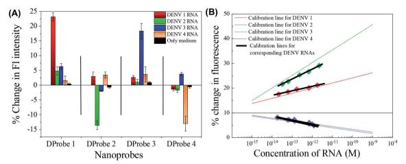
Fig. 7 (A) Comparative analysis of all four nanoprobes in the presence of all four types of DENV RNA serotypes. (B) Quantification of the dengue RNA isolated from DENV culture fluid. Intensities found from the fluorescence of each sample; ◆ Dengue 1, ◆ Dengue 2, ◆ Dengue 3 and ◆ Dengue 4, quantified from their calibration lines obtained in buffer solution. The black calibration lines are plotted from the RNA concentration.
