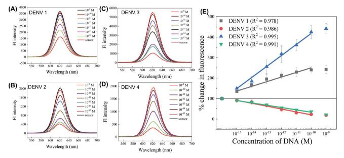
Fig. 6 (A–D) Concentration-dependent fluorescence changes of the CdSeTeS-dsDNA-AuNP nanocomposites in the presence of the target analyte DENV ssDNA of all four serotypes in the concentration range of  $10^{-15}$  to  $10^{-9}$  M. (E) Calibration curves for all four DENV serotypes.
