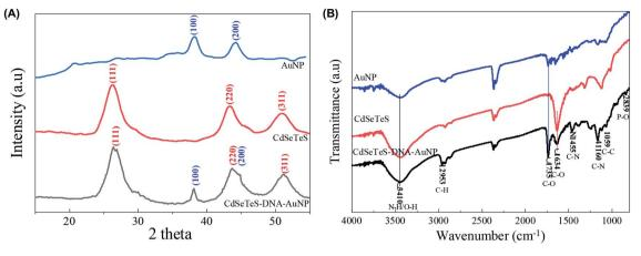
Fig. 3 Characterization of AuNP, CdSeTeS QDs and CdSeTeS-dsDNA-AuNP nanocomposites. XRD patterns (A) and FTIR spectra (B).
