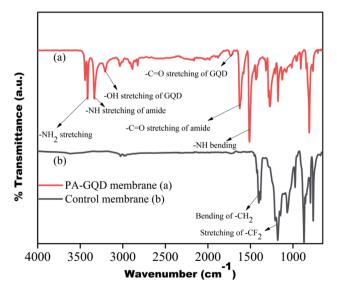
Fig. 8 FTIR spectrum of control and PA-GQD membranes.
