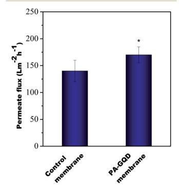
Fig. 11 Pure water flux of all samples. Flux was performed in triplicate, and \* indicates statistical significance with p < 0.05 analyzed with Bonferroni post-hoc analysis.
