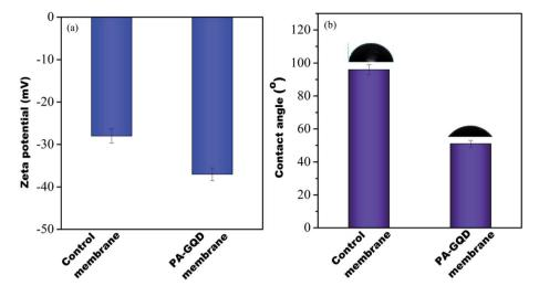
Fig. 10 Zeta potential (a) and contact angle (b) of control and PA-GQD membranes
