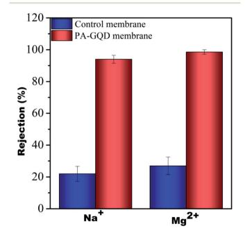
Fig. 14 Salt rejection performance of control and PA-GQD membranes.
