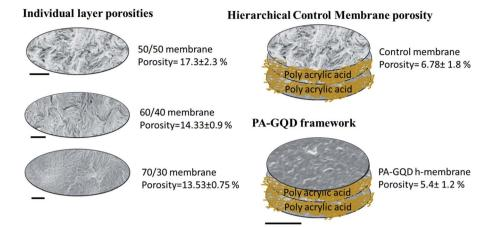
Fig. 15 Role of individual layers and their arrangement in selectively remediating dye pollutants and salt ions. The scale bar indicated is 2 µm.
