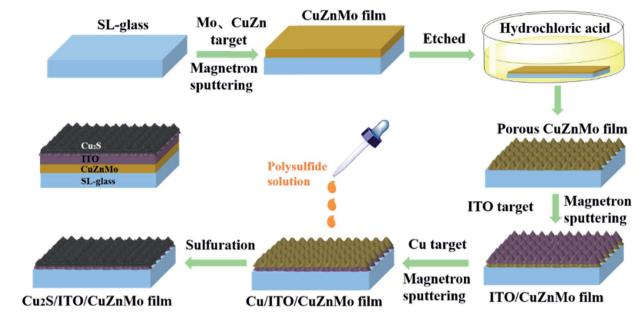
Fig. 1 Schematic diagram for preparing multilayer Cu<sub>2</sub>S(t)/ITO/CuZnMo functionalized film CEs.
