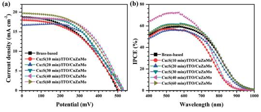
Fig. 7 (a) J-V curves and (b) IPCE spectra of QDSCs using different multilayer Cu<sub>2</sub>S(t)/ITO/ZnMo functional films and brass-based CEs.
