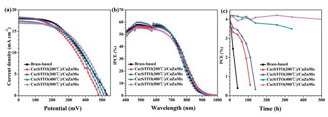
(a) J-V curves and (b) IPCE spectra of QDSCs using different multilayer  $Cu_2S/ITO(T)/CuZnMo$  functional films and brass-based CEs, and (c) PCE stability of QDSCs assembled with different CEs
