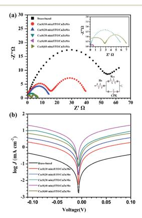
Fig. 8 (a) EIS Nyquist diagram; (b) Tafel polarization curves of symmetric cells based on multilayer Cu<sub>2</sub>S(t)/ITO/CuZnMo functional films and brass-based CEs.
