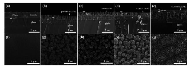
Fig. 3 SEM micrographs of surface and cross-section of (a and f) CuZnMo conductive film, (b and g) porous CuZnMo conductive film, (c and h) porous ITO/CuZnMo film, (d and i) Cu/ITO/CuZnMo film, (e and j) Cu<sub>2</sub>S/ITO/CuZnMo film.
