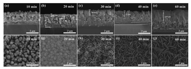
Fig. 6 SEM micrographs of surface and cross-section of multilayer Cu<sub>2</sub>S(t)/ITO/CuZnMo functional film prepared at different Cu sputtering times: (a and f) 10 min, (b and q) 20 min, (c and h) 30 min, (d and i) 40 min, (e and j) 60 min.
