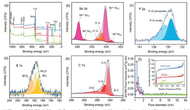
Fig. 4 (a) XPS survey of SbPO<sub>4</sub>/BC<sub>x</sub>, Sb/BC<sub>x</sub> and Sb/C, and the fitted Sb 3d signal (b), P 2p signal (c), B 1s signal (d), and C 1 s signal (e) for the SbPO<sub>4</sub>/BC<sub>x</sub> composite. (f) NLDFT adsorption pore size distribution plots (the inset presents N<sub>2</sub> adsorption-desorption isotherm curves) of the SbPO<sub>4</sub>/BC<sub>x</sub>, Sb/BC<sub>x</sub> and Sb/C samples.
