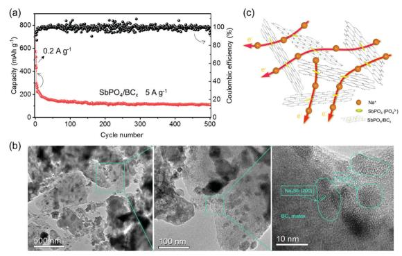
Fig. 6 (a) Cycling performance of the SbPO<sub>4</sub>/BC<sub>x</sub> electrode at 5 A  $q^{-1}$  after three cycles at 0.2 A  $q^{-1}$ . (b) TEM images of the SbPO<sub>4</sub>/BC<sub>x</sub> electrode after 500 cycles. (c) Proposed mechanism of the SbPO<sub>4</sub>/BC<sub>x</sub> composite during the sodium storage processes
