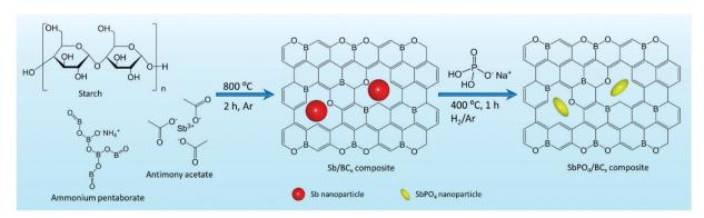
Fig. 1 Schematic illustration of the preparation process for the SbPO<sub>4</sub>/BC<sub>x</sub> composite.
