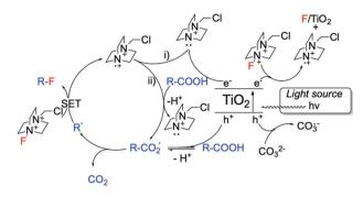
Scheme 15 Proposed reaction mechanism for TiO2-photocatalysed decarboxylative fluorinations. 102 Scheme adapted with permission from ref. 102 (American Chemical Society, https://pubs.acs.org/doi/10.1021/ acscatal.8b02844)
