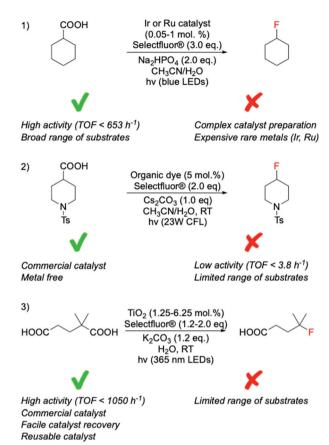
Scheme 9 Comparison of photocatalytic fluorination of carboxylic acids mediated by catalysts of different nature; (1) transition metal complexes, 99,100 (2) organic dyes, 101 and (3) heterogenous catalysts. 102 CLF = compact fluorescent lamp, LED = light-emitting diode.
