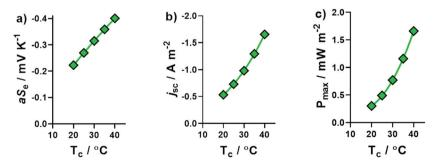
Fig. 4 Plots showing the significant effect different applied  $T_c$  values have upon the thermogalvanic properties of the  $[Fe(SO_4)_2]^{-/2-}$  system, as quantified by the (a)  $aS_e$ , (b)  $j_{SC}$ , and (c)  $P_{max}$ . For all measurements  $\Delta T = 10$  K, applied  $T_h = T_c + 10$  °C, and applied  $T_c$  is indicated by the x-axis. Second order polynomial lines of best fit have been added to guide the eye of the reader, and are not intended to model the data.
