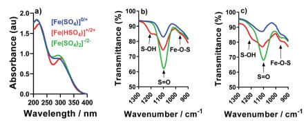
Fig. 5 Showing (a) UV-Vis spectra and (b and c) IR spectra of dilute analogues of the  $[Fe(SO_4)]^{0/+}$  (blue lines),  $[Fe(HSO_4)]^{+/2+}$  (red lines) and  $[Fe(SO_4)]^{2/-}$  (green lines) systems. Note that all used 0.03 M iron sulphate in a single oxidation state, plus 0.075 M Na<sub>2</sub>SO<sub>4</sub>/NaHSO<sub>4</sub> (as applicable); (a) and (c) used 0.03 M iron(III) sulphate.
