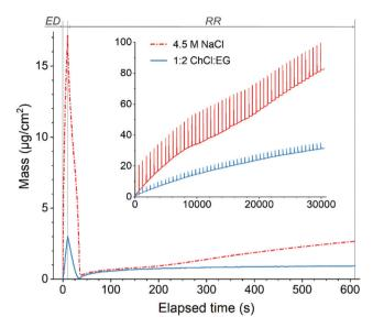
Fig. 2 Variation of mass during one EDRR cycle (10 s ED + 600 s RR) in aqueous 4.5 M NaCl solution and 1:2 ChCl:EG (60 mM Cu, 0.5 mM Au, T = 25 °C). Inset: mass change throughout 50 EDRR cycles.
