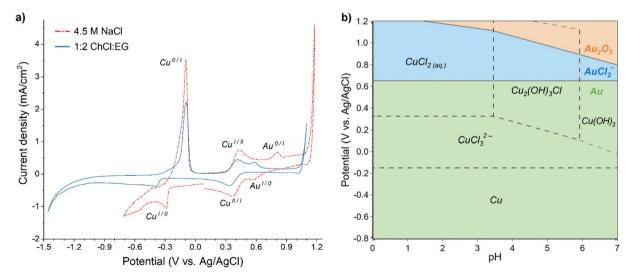
Fig. 1 (a) Cyclic voltammogram of 60 mM Cu + 0.5 mM Au in aqueous 4.5 M NaCl and 1:2 ChCl: EG solutions, scan rate 20 mV s<sup>-1</sup>. (b) Pourbaix diagram for aqueous Au-Cu-Cl system at 25 °C ([Au] = 0.5 mM, [Cu] = 60 mM, [Cl] = 4.5 M), generated in HSC Chemistry 10 software.
