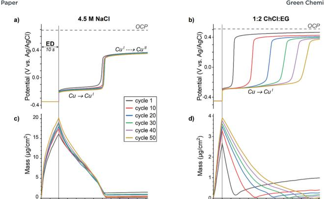
Fig. 4 Measured potential (a, b) and mass change (c, d) during first minutes of EDRR cycles in aqueous 4.5 M NaCl solution (left) and in 1:2 ChCl: EG (right).
