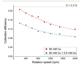
Fig. 5 Apparent collection efficiency of the ring-disk electrode as a function of rotation speed in aqueous 4.5 M NaCl solution.
