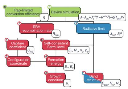
Fig. 1 Diagram for the calculation of trap-limited conversion efficiency. The dependent calculations are connected by lines. For each numbered step, the calculated quantities are appended. The red and blue boxes represent calculations for radiative and nonradiative electron–hole recombination, respectively. The combined device simulations are marked in green. The corresponding physical processes are detailed and illustrated in the ESI.†
