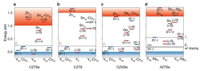
Fig. 4 Defect levels of native defects. Donor (red) and acceptor (blue) levels of native point defects of Cu<sub>2</sub>ZnSnSe<sub>4</sub> (a), Cu<sub>2</sub>ZnSnSe<sub>4</sub> (b), Cu<sub>2</sub>ZnGeSe<sub>4</sub> (c), and Aq<sub>2</sub>ZnSnSe<sub>4</sub> (d). Blue and red bands represents valence and conduction bands, respectively. Fermi levels are shown in gray lines. The black line in d represents the Fermi level of  $Ag_2ZnSnSe_4$  with a doping density of  $10^{20}~cm^{-3}$
