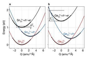
Fig. 5 Configuration coordinate diagram for carrier capture. Potential energy surfaces for the vibrations of Sn<sub>Zn</sub> (2+/+) in Cu<sub>2</sub>ZnSnSe<sub>4</sub> (a) and  $Ge_{Zn}$  (2+/+) in  $Cu_2ZnGeSe_4$  (b). The solid circle represents the relative formation energy calculated using DFT, and the line is a spline fit.  $E_{\rm b}$ represents the electron-capture barrier.
