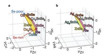
Fig. 3 Growth condition. Calculated phase diagrams of Cu<sub>2</sub>ZnSnSe<sub>4</sub> (a) and  $Ag_2ZnSnSe_4$  (b) where  $\mu_i$  = 0 represents the chemical potential of element iin its elemental state. Each plane represents a phase boundary with the secondary phase. Blue and red circles indicate Se-poor and Se-rich conditions, respectively
