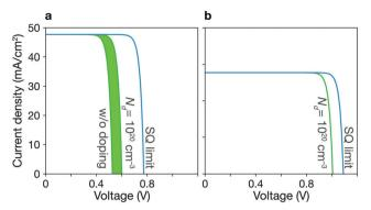
Fig. 7 Current-voltage simulation. J-V curves for CZTSe (a) and AZTSe (b) solar cells based on the properties of the bulk absorber materials and not including interfacial processes. Green lines represent the TLCs with various doping concentrations up to  $10^{20}$  cm<sup>-3</sup>. The SQ limit is shown in the blue curve.
