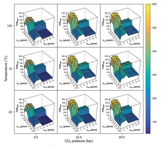
Fig. 2 Trellis plot of the random forest predictions  $\hat{f}(T, p_{H_2}, p_{CO_2}, t, n_{cat}, n_{add}, V)$  with  $p_{H_2} = 90$  bar, t = 18 h and V = 0.5 mL. Note the difference of max(TON<sub>DMM</sub>) in the experimental data (Table 1, entry 8) and the model. The RF values are predictions causing the range of the z-axis to be smaller than the range of the empirical data.
