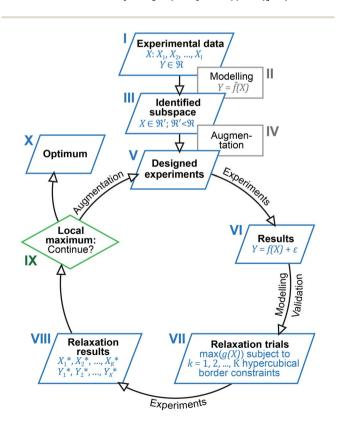
Fig. 1 Outline of the algorithm-based workflow combining experimental data analysis, DoE and optimisation.
