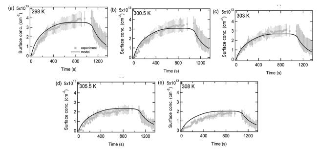
Fig. 6 Adsorbed limonene concentrations on SiO<sub>2</sub> as a function of time at an equilibrium pressure of 14 mTorr and at five different temperatures (a) 298 K, (b) 300.5 K, (c) 303 K, (d) 305.5 K, and (e) 308 K. A 20% error has been assumed for the adsorption part of the graphs while for the desorption part of the graphs a range of values are shown, representing experimental uncertainty described previously
