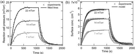
Fig. 5 (a) Temporal evolution of limonene pressures in the reaction cell and (b) adsorbed limonene concentrations on SiO<sub>2</sub> as a function of time for three different limonene equilibrium pressures, 7 (light grey), 14 (dark grey) and 22 (black) mTorr. Error bars represent the standard deviation between triplicate replicates of the same experiment.
