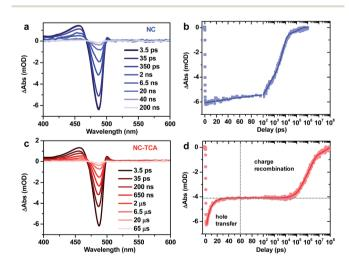
Fig. 2 (a) TA spectra of NCs probed at indicated time delays following excitation with a 340 nm pulse (with  $\langle N \rangle \sim$  0.07). (b) TA kinetics of NCs probed at an exciton bleach (XB) center of  $\sim$ 487 nm (blue squares) and its multi-exponential fit (blue solid line). (c and d) Similar plots to (a) and (b) for NC–TCA complexes.
