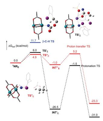
Fig. 12 Calculated free energy profile for the reactivity of  $NR_E$  at the PBE/BS2 level of theory (the relative free energies ( $\Delta G_{sol}$ , kcal mol<sup>-1</sup>) in ethyl acetate are provided). (Different atom styles are used for clarity.)
