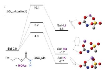
Fig. 2 Calculated free energy profile for the formation of the potassium, sodium and lithium N-mesyloxycarbamate salts for A at the PBE/BS2 level of theory (the relative free energies ( $\Delta G_{\rm sol}$ , kcal  ${\rm mol}^{-1}$ ) in ethyl acetate are provided). (Different atom styles are used for clarity.)
