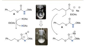
Scheme 3 Formation of the potassium and sodium N-mesyloxvcarbamate salt from A.
