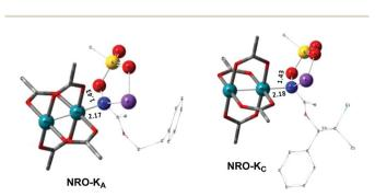
Fig. 4 Optimized structures of the NRO-K of A and C. (Sulfur atom: yellow; oxygen atom: red; nitrogen atom: blue; rhodium atom: aqua.) Key bond distances (Å) are indicated. (Different atom styles are used for clarity.)
