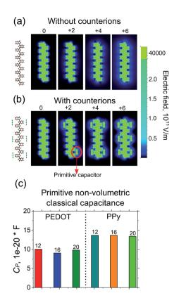
Fig. 4 Electric field intensity distribution in PEDOT oligomers of the length N=12 (a) without counterions, (b) with counterions for different total charges on the chains, Q=0, +2, +4, +6. (c) The primitive capacitance for PEDOT and PPy oligomers of different lengths.
