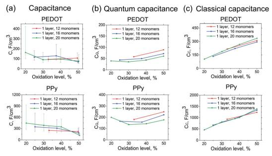
Fig. 2 Calculated capacitance of PEDOT and PPy for oligomers of different lengths (N = 12, 16, 20) as a function of the oxidation level. (a) Total capacitance  $C_C$ , (b) quantum capacitance  $C_C$ , (c) classical capacitance  $C_C$ . Upper and lower panels show results for PEDOT and PPy respectively.
