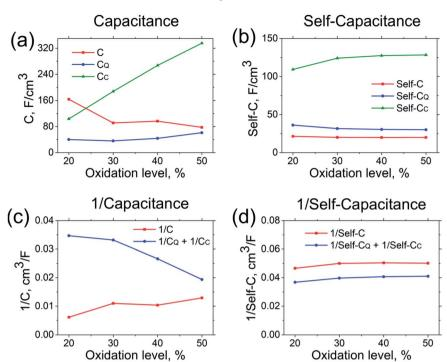
Fig. 3 Capacitance and self-capacitance of PEDOT (left and right panels respectively). (a) and (b) show the total capacitance  $C_C$ , quantum capacitance  $C_C$ , and classical capacitance  $C_C$ . Figures (c) and (d) compare 1/C and  $1/C_C$  according to eqn (8). Results correspond to the PEDOT oligomers of the length N=20.
