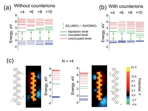
Fig. 5 Evolution of the electronic structure of PEDOT chains as the total charge of the chains increases, Q = +4, +6, +8, +10; (a) chain without counterions; (b) chain with counterions. (c) Electronic structure and potential distributions for two representative PEDOT chains with the same charge (Q = +4), but with a different configuration of counterions (shown in the inset).
