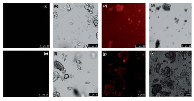
Fig. 4 Confocal using laser source and bright field images of the biosorbent after Cr(vI) adsorption (a and b) without RBH (c and d) with RBH (e and f) without RF (g and h) with RF.
