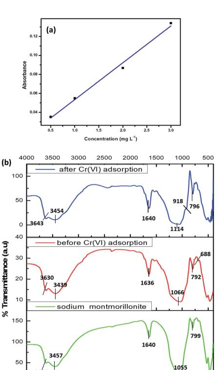
Fig. 1 (a) Calibration graph of Cr(vi) (b) FTIR of sodium montmorillonite, biosorbent before and after Cr(vi) adsorption.
