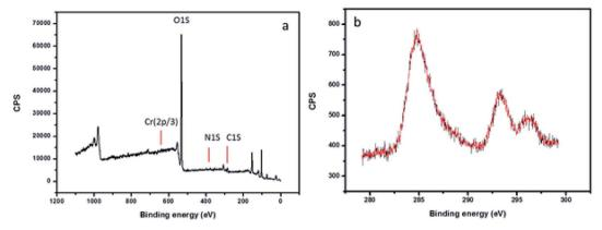
Fig. 3 XPS spectra of the biosorbent after Cr(vi) adsorption (a) survey scan spectra (b) high resolution spectra of C 1s.
