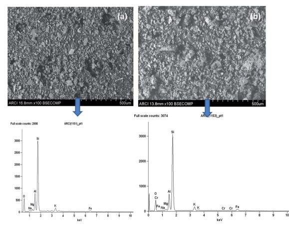
Fig. 2 SEM and EDAX images of the biosorbent (a) before Cr(vi) adsorption (b) after Cr(vi) adsorption.
