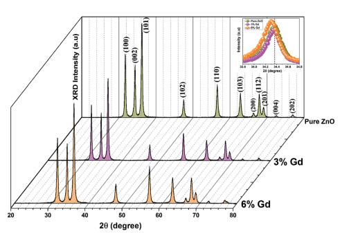
Fig. 1 X-ray diffraction patterns of pristine and Gd-doped ZnO-NRs annealed at 400 °C for 1 h. The X-ray diffractograms show that the prepared samples are polycrystalline with hexagonal wurtzite phase. The inset shows the shift of the diffraction peak along (002) plane at varying doping concentrations
