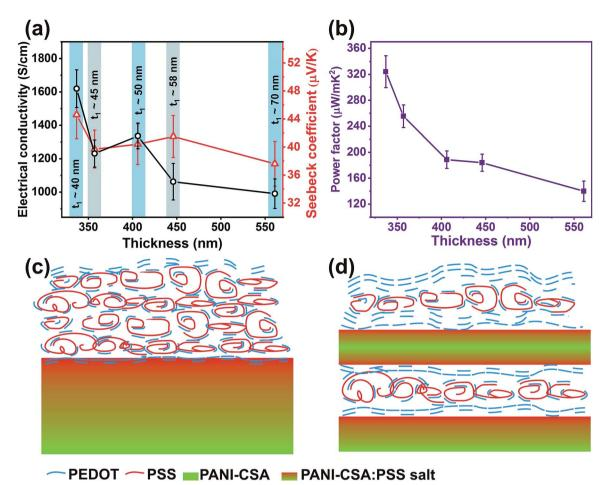
Fig. 5 (a) The electrical conductivity and Seebeck coefficients, (b) power factor of the PEDOT:PSS/PANI-CSA ML thin films at different layer thickness. The  $t_1$  in the figure shows the thickness of one PEDOT:PSS/PANI-CSA layer. (c and d) Schematics of the PEDOT:PSS/PANI-CSA ML thin films at different thickness. When the thickness of each layer decreases, the TE performances are enhanced through the removal of PSS from the PEDOT:PSS layer.
