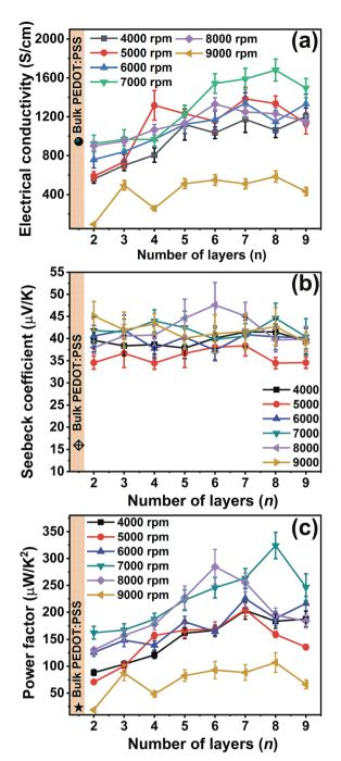
Fig. 2 (a) The electrical conductivity, (b) the Seebeck coefficient and (c) the power factor of PEDOT:PSS/PANI-CSA ML thin films deposited with respect to the number of layers and at various spin speed.
