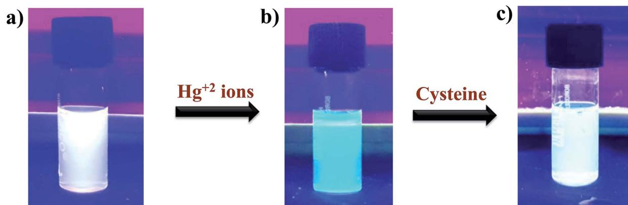
Fig. 6 Digital images of (a) WLEM; (b) WLEM with Hg<sup>2+</sup>; and (c) WLEM with Hg<sup>2+</sup> ions and Cys under UV light ( $\lambda_{\text{ex}} = 365 \text{ nm}$ ).
