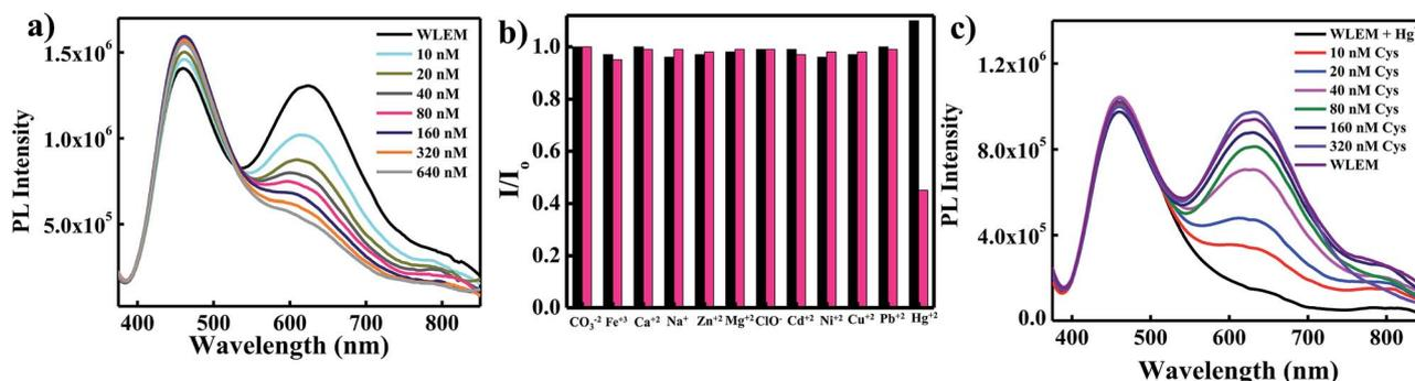
Fig. 5 (a) PL spectra of WLEM upon addition of different concentration of  $\text{Hg}^{2+}$  ions; and (b) change in PL intensity of Si QDs (black) and Au NCs (pink) in the WLEM upon addition of different ions; and (c) PL spectra of WLEM having  $\text{Hg}^{2+}$  ions with different concentration of Cys.
