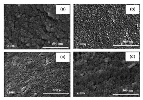
Fig. 5 PEDOT:PSS surface morphology at the EDOT:  $Na_2S_2O_8$  mole ratio of 1:1 and at various EDOT: PSS weight ratios: EDOT: PSS weight ratio of (a) 1:1, (b) 1:5, (c) 1:11 and (d) 1:13.
