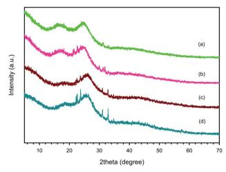
Fig. 2 XRD spectra of PEDOT:PSS at the EDOT:  $Na_2S_2O_8$  mole ratio of 1:1 and at various EDOT: PSS weight ratios: (a) EDOT: PSS weight ratio of 1:1, (b) EDOT: PSS weight ratio of 1:5, (c) EDOT: PSS weight ratio of 1:11, and (d) EDOT: PSS weight ratio of 1:13.
