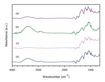
Fig. 1 FTIR spectra of PEDOT:PSS at the EDOT: PSS weight ratio of 1:11 and EDOT: Na<sub>2</sub>S<sub>2</sub>O<sub>8</sub> mole ratio of 1:2 with various surfactant types: (a) no surfactant, (b) CTAB (2.5CMC), (c) SDS (2.5CMC), and (d) Triton X-100 (2.5CMC).
