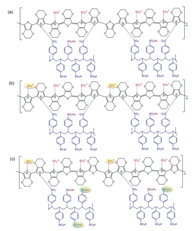
Scheme 3 Proposed structure of PEDOT:PSS at the EDOT: PSS weight ratio of 1:11 and at various EDOT: Na<sub>2</sub>S<sub>2</sub>O<sub>8</sub> mole ratios: at an  $EDOT: Na_2S_2O_8$  mole ratio (a) lower than 1:2, (b) 1:2, where  $SO_4^{2-}$  acts as a secondary dopant and (c) higher than 1:2, where a higher PSSNa amount is generated.
