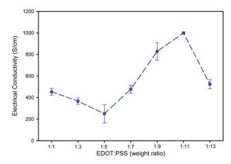
Fig. 8 Electrical conductivity of PEDOT: PSS at the EDOT: Na<sub>2</sub>S<sub>2</sub>O<sub>8</sub> mole ratio of 1:1 and at various EDOT: PSS weight ratios.
