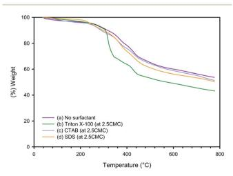
Fig. 7 TGA spectra of PEDOT:PSS at the EDOT: PSS weight ratio of 1:11 and EDOT: Na<sub>2</sub>S<sub>2</sub>O<sub>8</sub> mole ratio of 1:2: (a) no surfactant, (b) Triton X-100 (2.5CMC), (c) CTAB (2.5CMC) and (d) SDS (2.5CMC).
