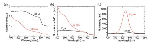
Fig. 4 Optical characterization of converted and reference 3D perovskite films on glass substrates. (a–b) UV-vis absorbance spectra without normalization (a) and with normalization at 840 nm (b), (c) steady-state PL spectra. Note that 3D\_ref and 3D\_conv as indicated in the figures denote the reference one-step coated and converted FAPbl<sub>3</sub> perovskites, respectively.
