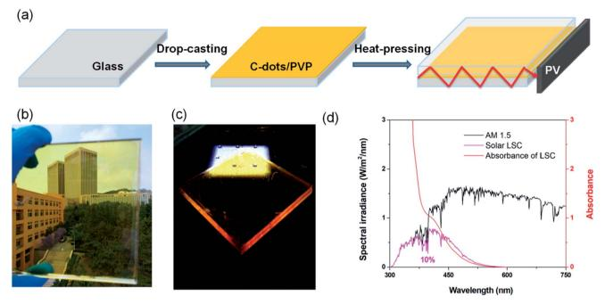
Fig. 3 (a) Scheme of the preparation process for laminated LSCs based on C-QDs. Photographs of the LSC under ambient (b) and one sun (100 mW cm $^{-2}$ ) illumination (c). LSC dimensions,  $10 \times 10 \times 0.9$  cm $^{3}$ . (d) Absorption and calculated solar absorption of the LSC and solar spectrum (AM 1.5G). The concentration of the C-QDs in PVP was calculated to be 2.5 wt% in PVP based on the data obtained by thermal gravimetric analysis (TGA).
