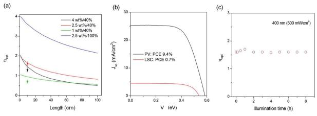
Fig. 5 (a) The calculated and measured external optical efficiency of LSCs based on C-QDs with a QY of 40% and different C-QD concentrations, and a QY of 100% with a concentration of  $3C_0$ . (b) J-V response of silicon PVs attached on the edge of the LSC under natural sunlight (62) mW cm<sup>-2</sup>). (c) The external optical efficiency of LSCs with a C-QD concentration of 2.5 wt% was measured using a power meter upon 400 nm illumination (500 mW cm<sup>-2</sup>).
