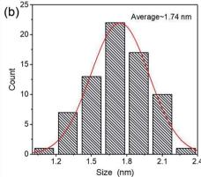
Fig. 1 (a) Representative TEM image of C-QDs. Insets are the HRTEM image of an individual C-QD and SAED pattern. (b) The size distribution of C-QDs.
