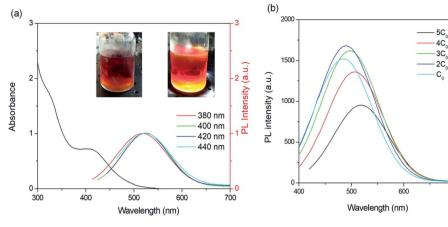
Fig. 2 Absorption and PL spectra of C-QDs dispersed in methanol solution. (b) PL spectra of C-QDs dispersed in methanol solution with different concentrations of C-QDs.  $C_0$  is 1 mg mL<sup>-1</sup>. The excitation wavelength is  $\lambda_{\rm ex} = 380-440$  nm for (a) and 380 nm for (b). The insets of (a) are the photographs of C-QDs dispersed in methanol under normal conditions (left) and upon simulated sunlight irradiation (100 mW cm<sup>-2</sup>).
