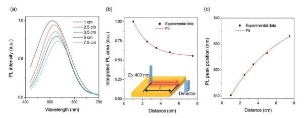
Fig. 4 (a) PL spectra measured at different optical paths (L) for the C-QD based LSCs. Integrated PL area (b) and emission peak positions (c) as a function of detection distance (L). The excitation wavelength is 380 nm. The inset of (b) is the scheme for distance-dependent PL measurement. The concentration of the C-QDs is 2.5 wt% in PVP.
