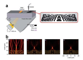
(a) Schematic of the experimental scheme (left) and a representative pattern of a relevant functional element (right). (b) Optimization of different structures that can focus Bloch surface waves behind the functional element. The optimized structures are shown in yellow. Reproduced with permission from ref. 125. Copyright 2018, Nature Publishing Group.
