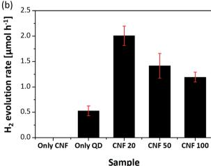
Fig. 6 (a) Energy band alignment diagram and proposed photocatalytic mechanism for CdSe–CNF. (b) Photocatalytic hydrogen evolution rates of the CNFs, CdSe QDs, and CdSe-CNFs in 0.25 M  $Na_2SO_3$  aqueous solution under visible light ( $\lambda \ge 420$  nm).
