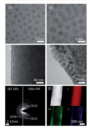
Fig. 3 (a) TEM image and (b) HRTEM image of CdSe QDs. (c) TEM image and (d) HRTEM image of CdSe-CNF 20. (e) SAED patterns of (left) CdSe QDs and (right) CdSe-CNF 20. (f) TEM-EDS mapping of CdSe-CNF 20
