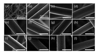
Fig. 2 SEM images of pristine CNFs in (a) low and (b) high magnification. SEM images of CNFs and CNFs coated with various kinds of QDs (20 mg mL $^{-1}$ ): (c) CdSe, (d) PbS, (e) InP, (f) CIS, (g) CdS, (h) InP/ZnS, (i) CIS/ZnS, (j) CdSe/ZnS, (k) CdZnSeS/ZnS, and (l) CdZnS/ZnS. Overall surface of the hybrid composite is uniform without aggregated QD particles.
