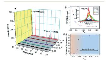
Fig. 3 (a) XRD  $\theta$ -2 $\theta$  scan results of films with different  $R_{Sr}$ . (b) Relationship between the FWHM of rocking curves of  $\alpha$ -quartz (100) and  $R_{Sr}$ . (c) Influence of  $R_{Sr}$  on the area coverage of dense  $\alpha$ -quartz. Those films were prepared with a withdrawal speed of 5 mm s<sup>-1</sup> under a relative humidity of 40% at 25 °C using Brij-58 as the surfactant. The annealing treatment was at 1000 °C for 300 minutes in an air atmosphere.
