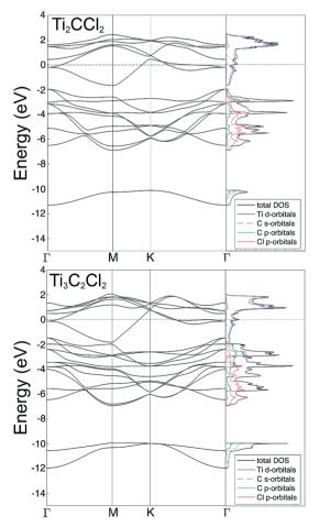
Fig. 3 Band structure and electronic density of states, resulting from the DFT calculations, for  $\text{Ti}_2\text{C}$  (top) and  $\text{Ti}_3\text{C}_2$  (bottom) with fcc coordinated Cl terminating the MXene surfaces.
