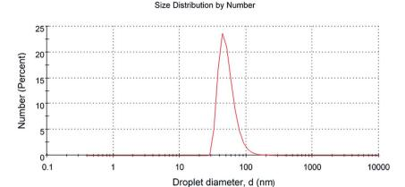
Fig. 4 Particle size distribution of CA (PHM3 algae) nanodots.
