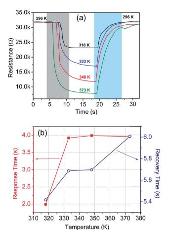
Fig. 8 (a) Sensor response at different temperatures in the  $296-373~\rm K$  temperature range, and (b) response and recovery time of the sensor at the corresponding temperatures.
