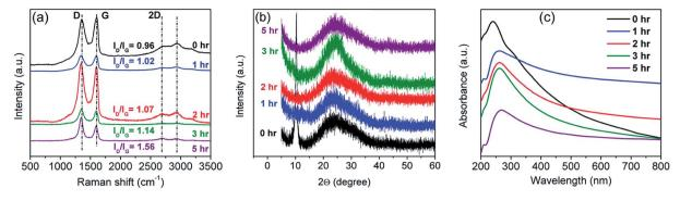
(a) Raman spectra, (b) XRD patterns, and (c) UV-Vis spectra of the prepared rGO sample as a function of reduction time.
