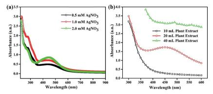
Fig. 2 UV-vis absorption spectra of Aq NPs synthesized at different concentrations of (a) AgNO<sub>3</sub> and (b) the plant extract.
