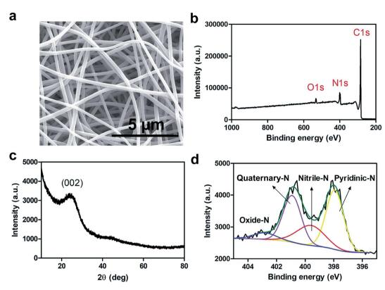
Fig. 1 SEM image of nCNFs produced at 800  $^{\circ}$ C (a). Survey XPS spectrum (b), XRD spectrum (c) and deconvoluted XPS spectrum (d) of N1s of nCNFs.
