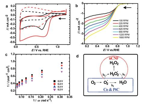
Fig. 3 CVs of oxygen reduction obtained at the Co100@nCNFs (red) and nCNFs (black) in N2 (dotted lines) and O2-saturated (solid lines) 0.1 M KOH solution at a scan rate of 10 mV s $^{-1}$  (a), RDE measurements at the Co100@nCNFs from 100 to 1600 rpm in O<sub>2</sub>-saturated 0.1 M KOH solution at a scan rate of 10 mV s<sup>-1</sup> (b), the Koutecky-Levich plot at 0.5, 0.4, 0.3, and 0.2 V vs. RHE (using data from (b)) (c), and schematic of the ORR mechanism (d).
