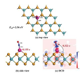
Fig. 5 Adsorption configuration (a) and (b) and DCD (c) of the Rh-MoSe<sub>2</sub>/NO system.
