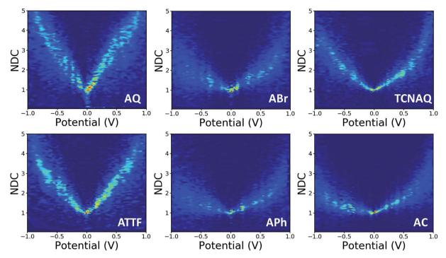
Fig. 5 Normalized differential conductance heatmaps for Au<sup>Mica</sup>/SAM//EGaln junctions comprising AQ, ABr, TCNAQ, ATTF, APh, and AC.
