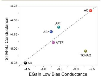
Fig. 6 Confrontation between the values of conductance obtained for single-molecule STM-BJ at 0.1 V (y-axis) and low-bias conductance extracted from Au<sup>Mica</sup>/SAM//EGaIn junctions (x-axis). Both data sets are presented on a logarithmic scale. The dashed line is intended as a guide to the eye for deviation from linearity
