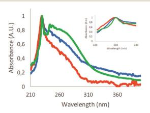
Fig. 2 Absorbance scans. Green: concentrated coffee cup lid particles; blue: expanded polystyrene foam filtered through 1.2  $\mu$ m filter; red: expanded polystyrene sample filtered through an additional 0.45  $\mu$ m filter. Inset: magnified polystyrene peak at around 230 nm. The absorbance scans were normalized against the highest value at around 230 nm in each sample.
