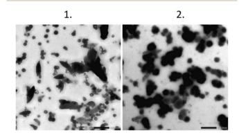
Fig. 4 TEM pictures of the particles. Scale bar is  $0.5~\mu m$ . Panel 1 is the  $1.2~\mu m$  filtered sample and panel 2 is the  $0.45~\mu m$  filtered sample.
