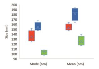
Fig. 5 Boxplot of NTA results. Red is expanded foam sample filtered through 1.2  $\mu m$  and then 0.45  $\mu m$  filter; blue is expanded foam sample filtered through 1.2  $\mu m$  filter; green is the coffee cup lid sample. Both the mode and mean size are shown. Whiskers show maximum and minimum values, crosses show mean values and horizontal lines show median values. Each treatment is based on the measurement of four individual samples.
