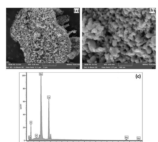
Fig. 7 (a) SEM secondary electron images of the CaMoO<sub>4</sub> synthesised at 500 °C showing: (a) a low magnification view of dense agglomerates of irregular-shaped particles; (b) details of (a) showing the rounded and elongated particles to be 50-250 nm in diameter with coarser scale pores between them; (c) EDS analysis showing the elemental composition of Ca, Mo, and O.
