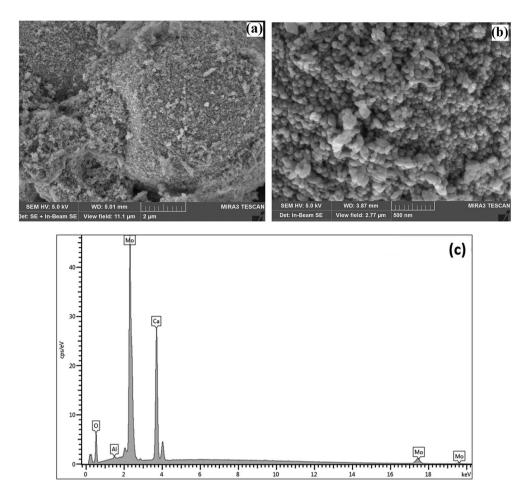
Fig. 6 SEM secondary electron images of the CaMoO<sub>4</sub> synthesised at 300 °C showing: (a) a low magnification view of dense agglomerates of small spherical particles; (b) details of (a) showing the rounded particles to be 120-100 nm in diameter with fine scale pores between them; (c) EDS analysis showing the elemental composition of Ca, Mo, and O.
