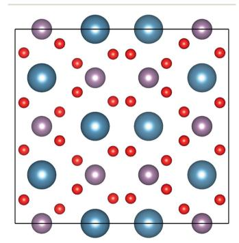
Fig. 2 Representation of the powellite-type crystal structures of CaMoO<sub>4</sub>. The atoms with blue, pink and red indicate Ca, Mo and O, respectively.
