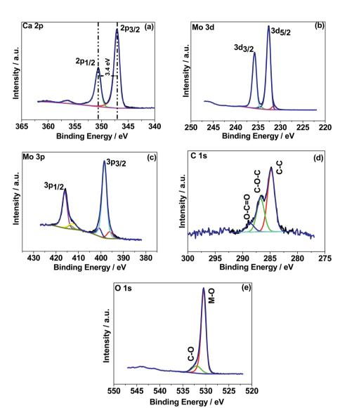
Fig. 5 X-ray photoelectron spectroscopy (XPS) spectra of CaMoO<sub>4</sub> synthesized at  $500 \,^{\circ}$ C. High resolution spectra for regions (a) Ca 1s, (b) Mo 3d, (c) Mo 3p, (d) C 1s, and (e) O 1s.
