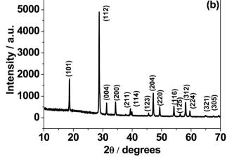
Fig. 1 X-ray diffraction (XRD) patterns of CaMoO<sub>4</sub> synthesized at: (a) 300 and (b) 500 °C. The lower temperature material displayed a much weaker pattern, suggesting that it was not as crystalline as the higher temperature counterpart.
