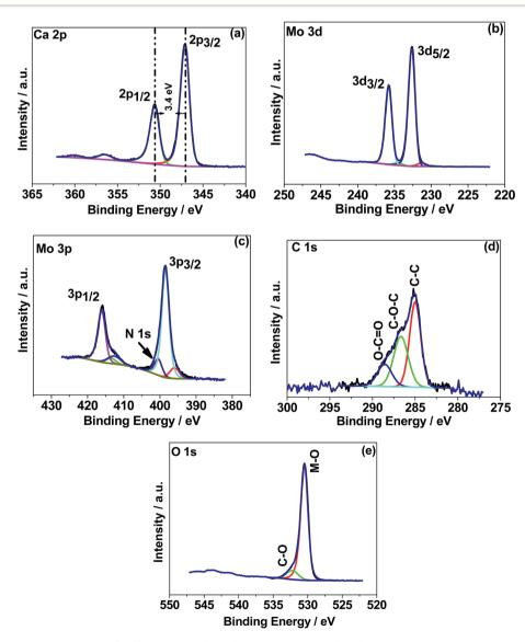
Fig. 4 X-ray photoelectron spectroscopy (XPS) spectra of CaMoO<sub>4</sub> synthesized at 300  $^{\circ}$ C. High resolution spectra for regions (a) Ca 1s, (b) Mo 3d, (c) Mo 3p, (d) C 1s, and (e) O 1s.
