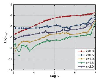
Fig. 9 Variation of AC conductivity with frequency of all the Ce<sup>3+</sup>-substituted YIG samples.
