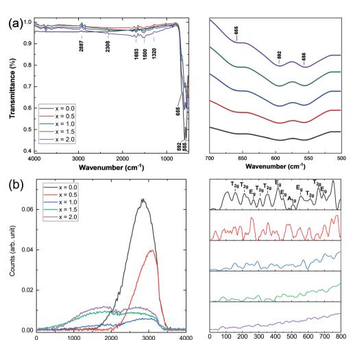
Fig. 3 (a) Infrared spectra and (b) Raman spectra of all the Ce<sup>3+</sup>-substituted YIG samples.
