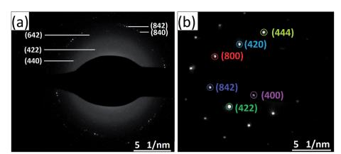
Fig. 6 SAED patterns of (a) polycrystalline YIG, x = 0.0, and (b) preferred (100) oriented single-crystalline Ce-YIG, x = 2.0.
