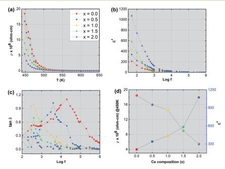
Fig. 8 (a) Variation of electrical resistivity ' $\rho$ ' as a function of temperature 'T', (b) variation of dielectric constant ' $\varepsilon$ ' as a function of logarithm of frequency 'log f', (c) variation in dielectric loss tangent 'tan  $\delta$ ' as a function of logarithm of frequency 'log f' and (d) variation of electrical resistivity '
