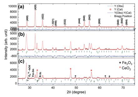
Fig. 2 Rietveld-refined XRD patterns of typical samples of  $Y_{3-x}$ Ce<sub>x</sub>Fe<sub>5</sub>O<sub>12</sub> powders annealed at 1150 °C for 10 h; (a) x = 0.0, (b) x = 1.0 and (c) x = 2.0.
