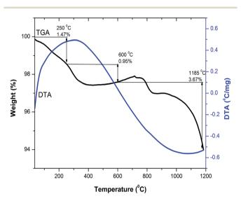
Fig. 1 Combined differential thermal analysis (DTA) and thermogravimetric analysis (TGA) curves of Y<sub>2</sub>Ce<sub>1</sub>Fe<sub>5</sub>O<sub>12</sub> composition.
