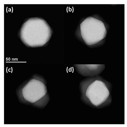
Fig. 2 Representative examples of  $Ag_2S/Ag$  particles at 8 min (a), 1 h (b), 8 h (c) and 24 h (d) of reaction time. The brighter central core is the Ag while the less intense regions nucleating along the particle vertices are  $Ag_2S$ . All particles are [111] oriented and the magnification is the same (see scale bar).
