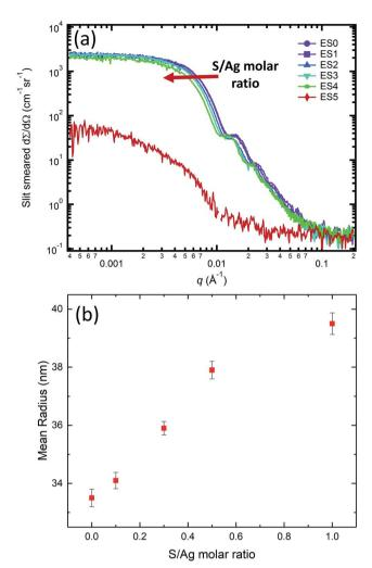
Fig. 6 (a) Scattering profiles of the *ex situ* AgNP suspension samples with S/Ag ratio of 0 (EB0), 0.1 (EB1), 0.3 (EB2), 0.5 (EB3), 1.0 (EB4), and 5.0 (EB5), respectively. (b) The dependence of mean size of the *ex situ* AgNP samples EB0-EB4 on the S/Ag molar ratio.
