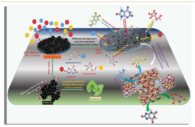
Scheme 3 Simple portrayal of the formation of pores in the PTPCNs, bulk diffusion of DA+, UA- and AA- at the PTPCNs/GCE, their interactions with the PTPCNs/GCE and electrochemical reactions of DA and UA through the surficial pores as well as the surface.
