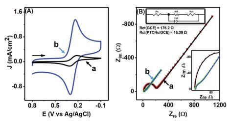
Fig. 6 (A) CVs and (B) EIS spectra of 5.0 mM K<sub>3</sub>[Fe(CN)<sub>6</sub>] in 1.0 M KCl at the GCE (a) and at the PTPCNs/GCE (b). The upper left side of (B) shows the Randel circuit, whereas the lower left inset shows the magnified EIS of the PTPCNs/GCE
