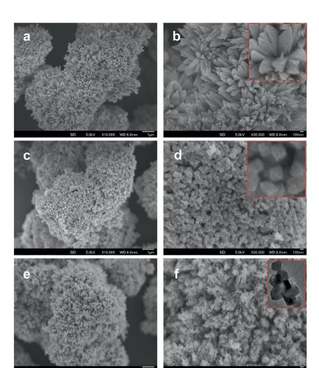
Fig. 2 SEM images: (a and b)  $[Co/Ni][OH]_2$ , (c and d)  $Co_3O_4/NiO-400$  °C, (e and f)  $Co_3O_4/NiO-600$  °C microsphere composites at low and high magnifications. Scale bars: 1  $\mu$ m in a, c, e; 100 nm in b, d, f.
