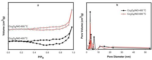
Fig. 6 Co<sub>3</sub>O<sub>4</sub>/NiO microspheres: (a) N<sub>2</sub> sorption isotherms; (b) micro- and mesopores distributions.
