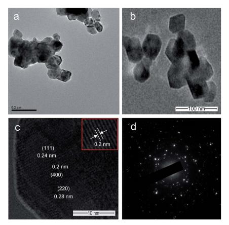
Fig. 3 TEM images of Co<sub>3</sub>O<sub>4</sub>/NiO-600 °C microspheres: (a and b) at high and low magnifications; (c) lattice plane; (d) SAED pattern.
