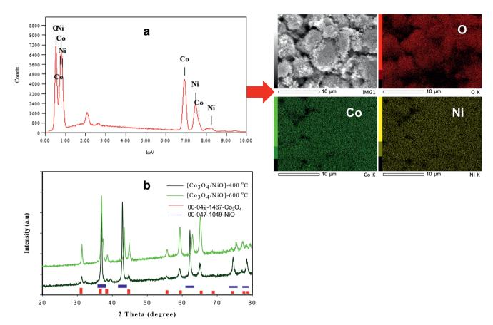
Fig. 4 Co<sub>3</sub>O<sub>4</sub>/NiO-600 °C microspheres: (a) EDS mapping; (b) XRD.
