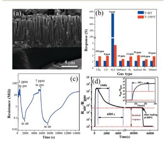
Fig. 4 (a) Cross-section SEM image of vertically aligned ZnO rods; (b) selectivity of the sensor at 25  $^{\circ}$ C and 250  $^{\circ}$ C; (c) response/recovery curves to 1 and 5 ppm H<sub>2</sub>S at room temperature.<sup>71</sup> Copyright 2015, Elsevier. (d) The response/ recovery curve at 50 ppm H<sub>2</sub>S gas at room temperature. <sup>101</sup> Copyright 2017,
