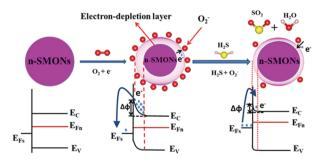
$E_C$ : bottom of conduction band;  $E_V$ : top of valence band;  $E_{Fn}$ : bulk Fermi level;  $E_{Fs}$ : surface Fermi level;  $\Delta \varphi$ : potential barrier;
