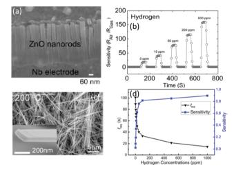
Fig. 9 (a) TEM image of vertical ZnO nanorods; (b) response/recovery curves of a vertical ZnO nanorod-based gas sensor versus different concentrations of H<sub>2</sub>. 190 Copyright 2012, Elsevier. (c) SEM images of  $\alpha$ -MoO<sub>3</sub> nanoribbons; (d) response values and times of an  $\alpha$ -MoO<sub>3</sub> nanoribbon-based gas sensor versus different concentrations of H<sub>2</sub>. 192 Copyright 2015, American Chemical Society.
